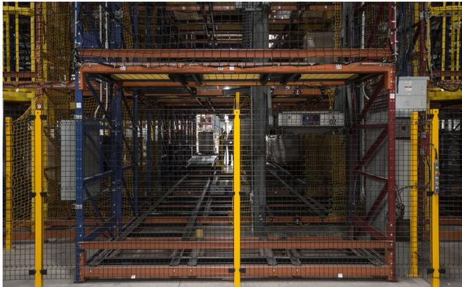
The AS/RS system conveyors, elevators, automated guided vehicles and variety of moving components required an innovative machine guarding solution to provide 24/7 safety, security and protection for employees and equipment. **Advance partnered with Husky Rack & Wire and utilized its Velox Machine Guarding system. Velox not only met the company's required internal security measures, but also exceeded regulatory safety standards.**
